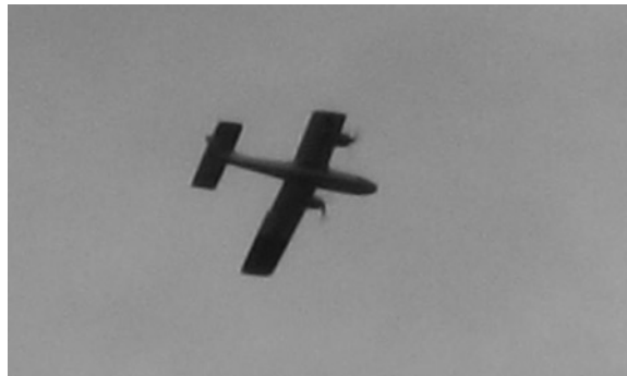
Fig. 5 GT Twinstar in autonomous flight after jettisoning 50% of its right wing in autonomous flight to simulate a severe structural damage.
